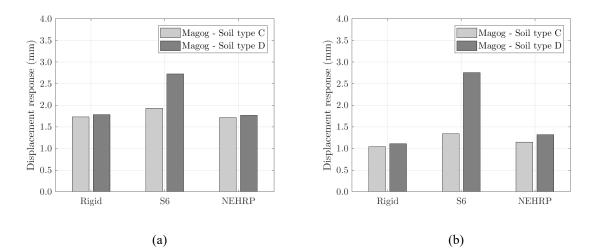
Figure 5. Superstructure displacement responses: (a) longitudinal direction and (b) transverse direction.
