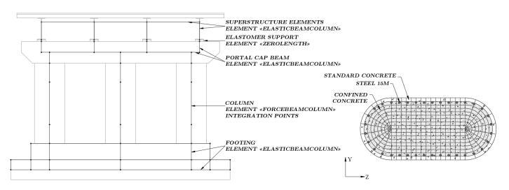
Figure 2. Discretization of the elements of the bridge bent and transversal section of a column.
