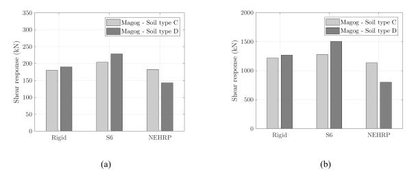
Figure 6. Shear responses at the base of the bridge bent: (a) longitudinal direction and (b) transverse direction.
