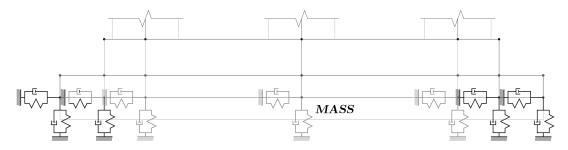
Figure 3. Foundation model for the bridge bent fo Chemin Roy Bridge (dampers are present only in the NEHRP model).
